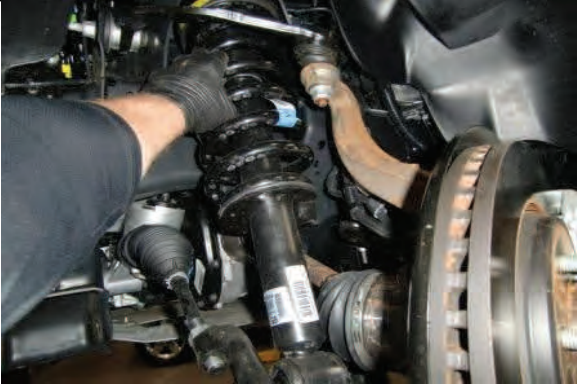
Remove strut assembly from vehicle
