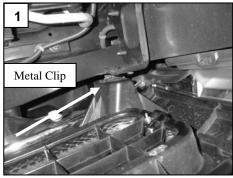
**STEP 2:** Test fit the grilles into the openings. Remove the radiator cover from the vehicle; then the four 10mm bolts along the top of the grille. The grille has metal clips along the bottom and center (1); these secure the grille to the core support. Use a slotted screwdriver to release the clips. Remove the grille. If you have purchased the lower grille; install grille now.
