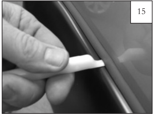
Using flat end of supplied Edge Trim Tool (Item 13), seat edge trim against flare by inserting straight end between edge trim and flare at one end. Next, slide around entire edge to the other end.
