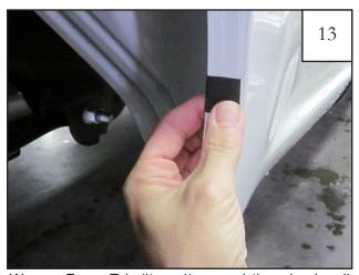
Wrap a Foam Tab (Item 4) around the wheel well sheet metal, centered over each of the upper four marks made in Step 15. Place a Mylar Tab (Item 7) at the mark made on the lower front of the wheel well (see step 14).
