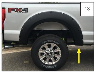
Start a supplied screw (Item 6) through the flare into the clip installed in Step19. Tighten all screws.
