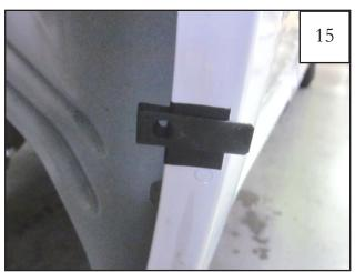
Install a Clip (Item 3) over each of the four Tabs (Item 4) placed over the upper 4 marks made in Step 16.
