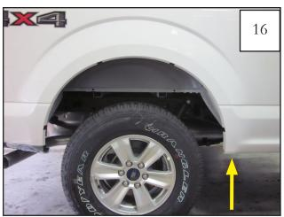
Install a supplied "S" clip (Item 5) over the mylar tab installed at the lower front of the rear wheel well.
