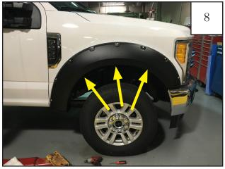
Position flare on fender, pressing inward on the flare, line up the flare mounting holes with the mounting clips on the inner piece. Install 3 Phillips Truss Screws (Item 2) through the flare and into the clips on the inner piece. Do not tighten. (3 locations)
