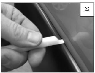
Using flat end of supplied Edge Trim Tool (Item 13), seat edge trim against flare by inserting straight end between edge trim and flare at one end. Next, slide around entire edge to the other end.
