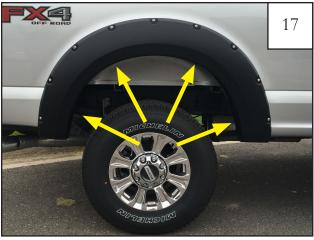
While holding flare to vehicle, start supplied screws (Item 2) through the four topmost mounting holes in flare and into the clips installed in Step 18.
