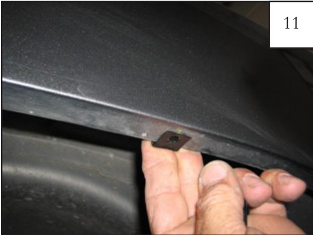
Center a supplied Clip (Item 1) over the upper two marks made in Step 9. Clips may need to be adjusted to align with holes in flare. Note: The raised collar on the Clip should face upward into the interior of the fender.
