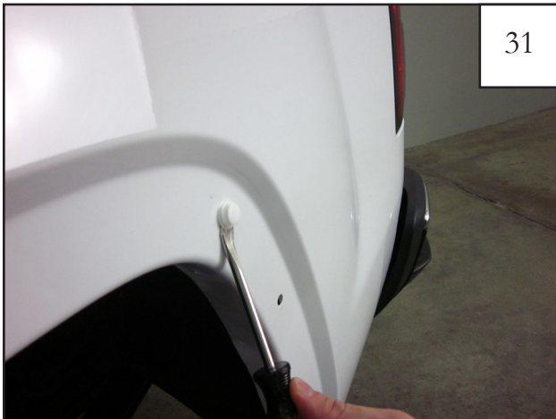
31 Use a pry tool to remove any remaining factory fasteners that may have stayed on the vehicle during the removal process.
