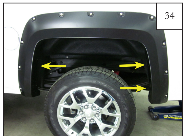
34 Hole locations to be marked for drilling.
