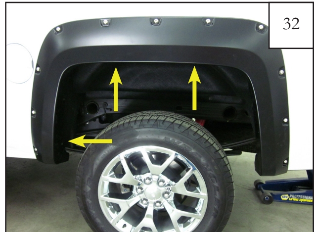
32 Hold rear flare up to wheel well to confirm fit. While holding flare on vehicle, install supplied screws (Item 2) into the 2 upper and 1 lower factory hole locations. Do not fully tighten at this time.
