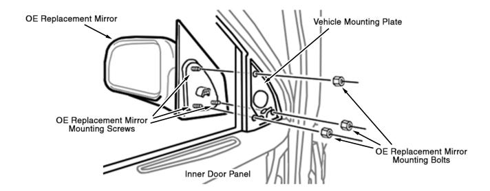
CIPA-USA, Inc. will not be responsible for damage to mirror, door, or any vehicle parts, components, or equipment due to improper removal or installation of OE Replacement mirrors. It is highly suggested to have a professional installer perform the installation.
