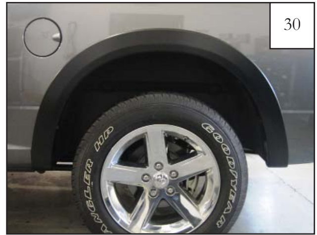
Completed rear flare installation.
