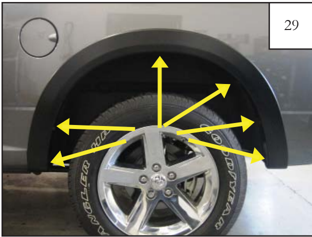
Press firmly on flare and tighten all screws.
