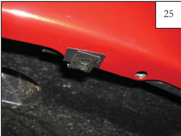
Install speed clip over plastic tab.
