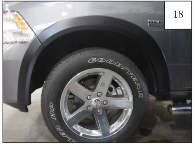
PLASTIC BUMPER ONLY: Completed front flare installation.
