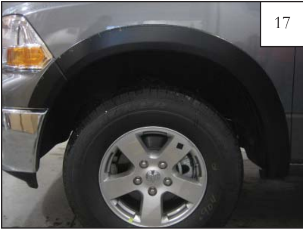
METAL BUMPER ONLY: Completed front flare installation.
