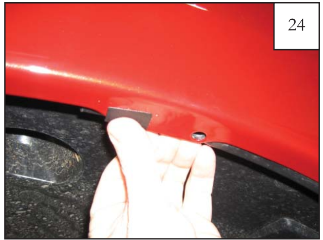
Install plastic tab over existing factory hole.
