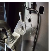
**STEP 6:** Unbolt the brake line at the frame and straighten out the bracket guide.
