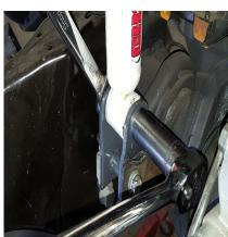
**STEP 10:** Install the new shock extender into the factory mount on the axle using the factory hardware. Next, install the shock into the extender and tightened using the provided hardware.
