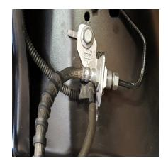
STEP 7: Rotate the brake line bracket 90 degrees NOTE: You will need to manipulate some bend out of the hard line in order to rotate the bracket. Rotating the bracket will allow the axle to droop out further and not pinch the brake line while doing so.
